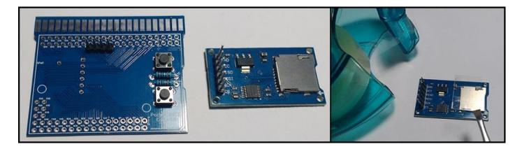
4.1- Cut leveled to PCB the remnants top and bottom Module SDcard pin bar:
